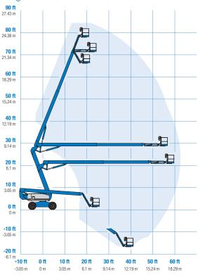
\* The metric equivalent of working height adds 2 m to platform height.
